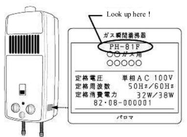
The above models of indoor gas fired water heaters have defective safety device which can fail to operate properly and may cause serious accident of taking your life due to incomplete combustion. Paloma Industries are committed to inspect, repair or replace any still in use for free. Please check your water heater and if it meets the saidmodel, ask to replace it with new water heater.
